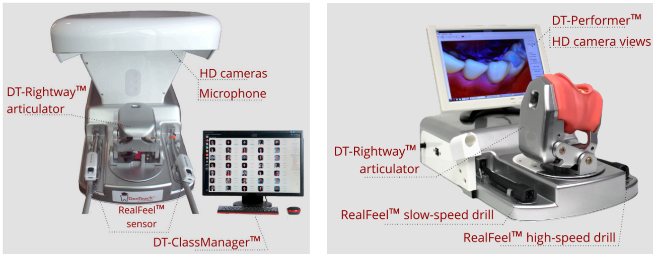
Figure 2. DenTeach comprises the DT-Instructor (instructor workstation) and DT-Student (student workstation) that communicate through a cloud-based communication channel.
