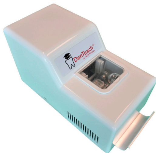
Figure 6. PrepScanner is an automated measuring device that provides fast, precise, and objective tooth preparation grading.
