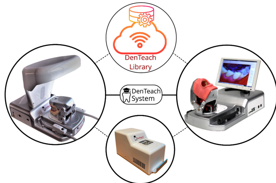
Figure 8. DenTech Library is the brain of the DenTech platform that connects data and information among the student workstations, the instructor workstation, and the scanner.
