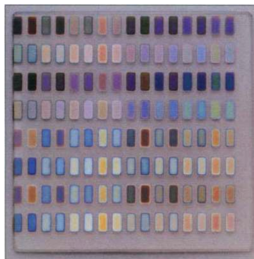
FIG. 41. A 128-member matrix array cuprate superconductor library, prior to sintering. Each site is 1 mm by 2 mm; the color of each is the natural color of reflected light from a white light source. The amorphous precursor layers are deposited using a series of shadow masks. Reproduced with permission from X. D. Xiang et al. , Science 268 , 1738 (1995). Copyright 1995 American Association for the Advancement of Science.
