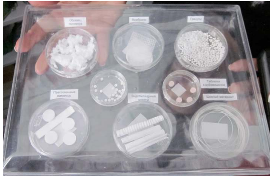
Figure 2: Examples of PHA matrices fabricated for medical use. Items such as meshes (top, middle) and fibers for sutures (bottom, right) show promise for surgical use. Pellets (middle and bottom, left) and microspheres (top, right) have been explored for drug delivery. Films (bottom, right) have uses in post-surgery recovery, as well as potential agricultural applications.
