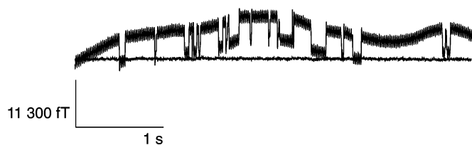
Fig. 18. Original and SSS reconstructed signal of one misbehaving magnetometer channel showing a step-like artifact signal and power line interference. The signal is from an empty room measurement.
