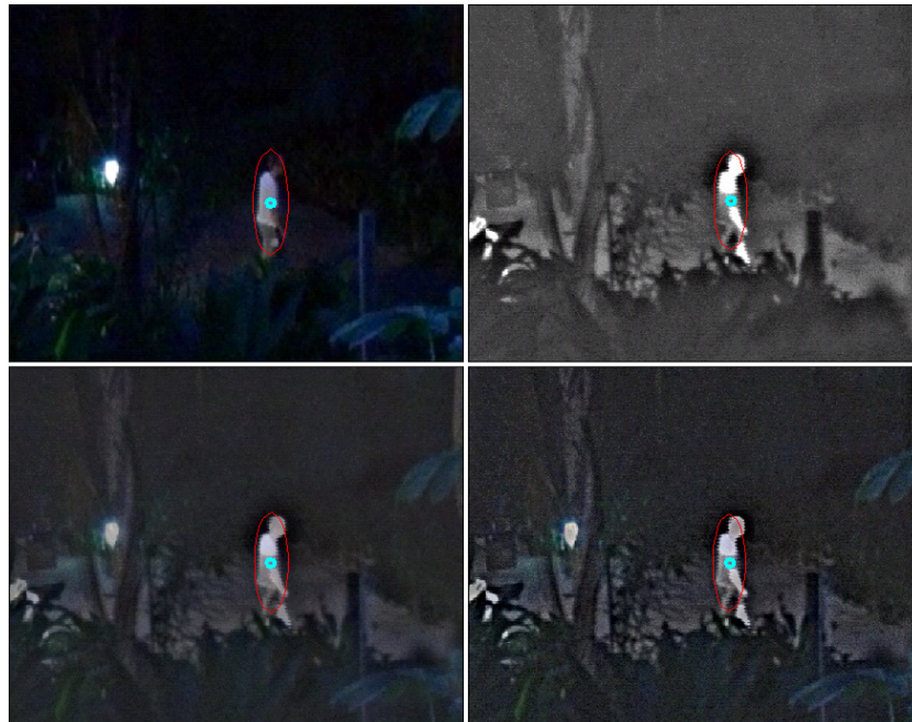
Figure 8: Tracking in an Eden sequence. Clockwise from top left the results correspond to: visible, infrared; DT-CWT fused and average fusion
