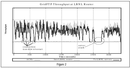
torn down and a new transfer started. This causes spikes in the data transmission rate, especially when all four files ended at approximately the same time. We also had a several minute period where one of the receiving servers had crashed and we had to reboot, and restart the transfer.
