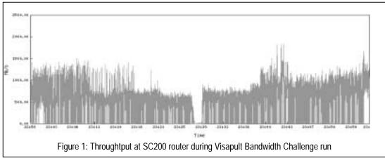
is common in high energy physics (HEP) applications. During the course of the contest, background DPSS *get* operations were run to use up the spare DPSS bandwidth (roughly 500 Mb/s) due to a bottleneck at Visapult's rendering engine. The DPSS obtained a peak of 1.48 Gb/s and sustained throughput of 582 Mb/s, as measured at the ingress router to the show floor.
