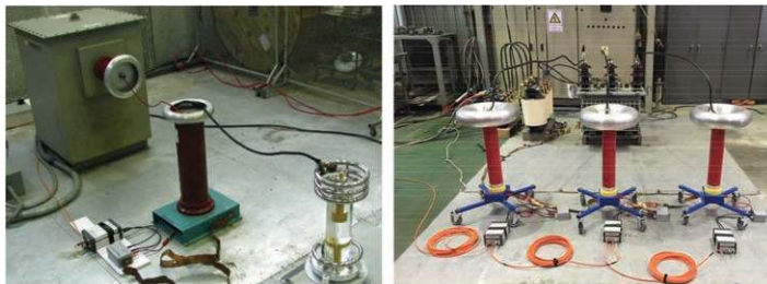
Figure 10 Test arrangement for PD in oil and transformer and measuring system.
