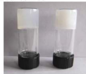
Fig. 20 Chemical structures of ligand 30 and photograph of hydrogels of 30b in ratios with \text{Pb}^{2+} of 1 : 0.3 (left) and 1 : 1 (right). Figure adapted from ref. 73 with permission.
