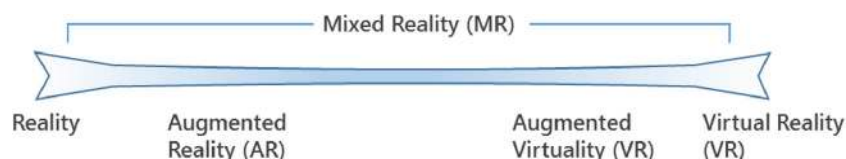
Fig. 2 Illustration of the reality-virtuality continuum. Augmented reality (AR) is a subset of the mixed-reality space between the two extremes of the continuum, with reality (i.e., a completely real environment) on one end and virtual reality (i.e., a completely virtual environment) on the other
