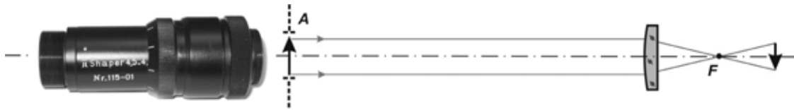
Fig. 3 Relay imaging of the \pi Shaper output aperture to the working plane.
