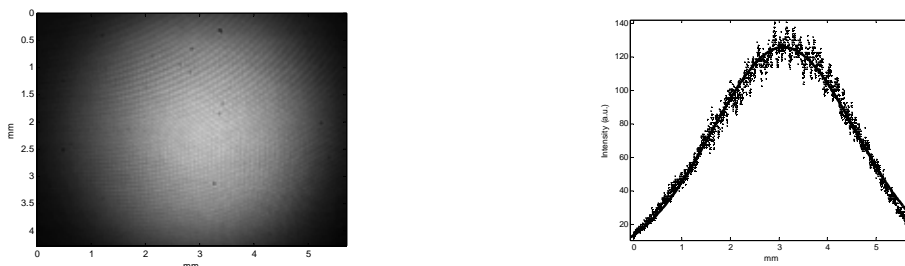
Fig. 7 Image (directly onto camera) and cross-section of input beam to \pi Shaper 6_6_VIS (E), 1/e^2 diameter = 5.9 mm.
