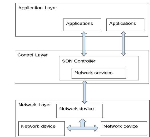
Fig. 2 A typical SDN architecture
