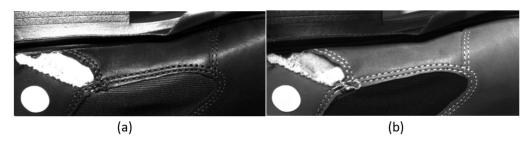
Figure 6. Comparison of 200 mm red light (a) and circular 100 mm IR light (b).
