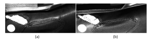
**Figure 5.** Demonstrating impact of position line 200 mm red light: ((**a**) light source placed above, (**b**) light source placed below).
