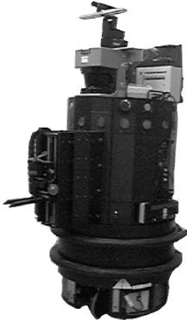
Figure D.1: Nomad200 platform called Asterix has 16 sonars and a PLS laser scanner. The upper body of the platform can rotate and thus the direction of the laser can be controlled.
