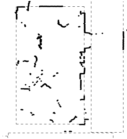
Figure 6.16: The result of combining two horizontal laser scans to give a 360° view of the living-room. Notice how the left and the lower walls are almost completely occluded when using a Scout robot with the sensor at 0.5 m above ground.
