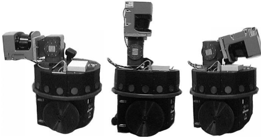
Figure D.2: The SuperScout Louie with a PTU mounted LMS. Using the PTU the direction of the laser scanner can be controlled. In the upright position the laser is 52 cm above ground.
