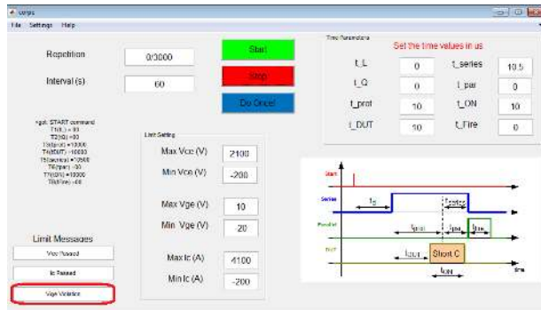
Fig. 6. Graphical User Interface (GUI) developed in MATLAB ® to perform repetitive short-circuit tests. A sample violation condition has been evidenced in the picture.
