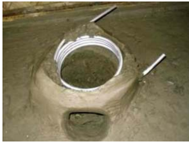
Fig. 2 Chulli purifier in the form of a coiled tube (Islam and Johnston 2006)
