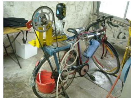
Fig. 16 Pedal powered UF system. Photo: Ramprasad V
