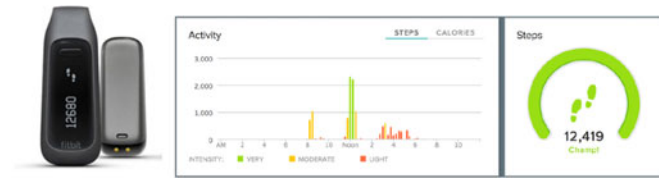
Fig. 1. The Fitbit one (left) was one of the wearable fitness tracking devices used for this study. Activity data are displayed on the Fitbit dashboard (fitbit.com) using time-ordered and aggregate representations (right).
