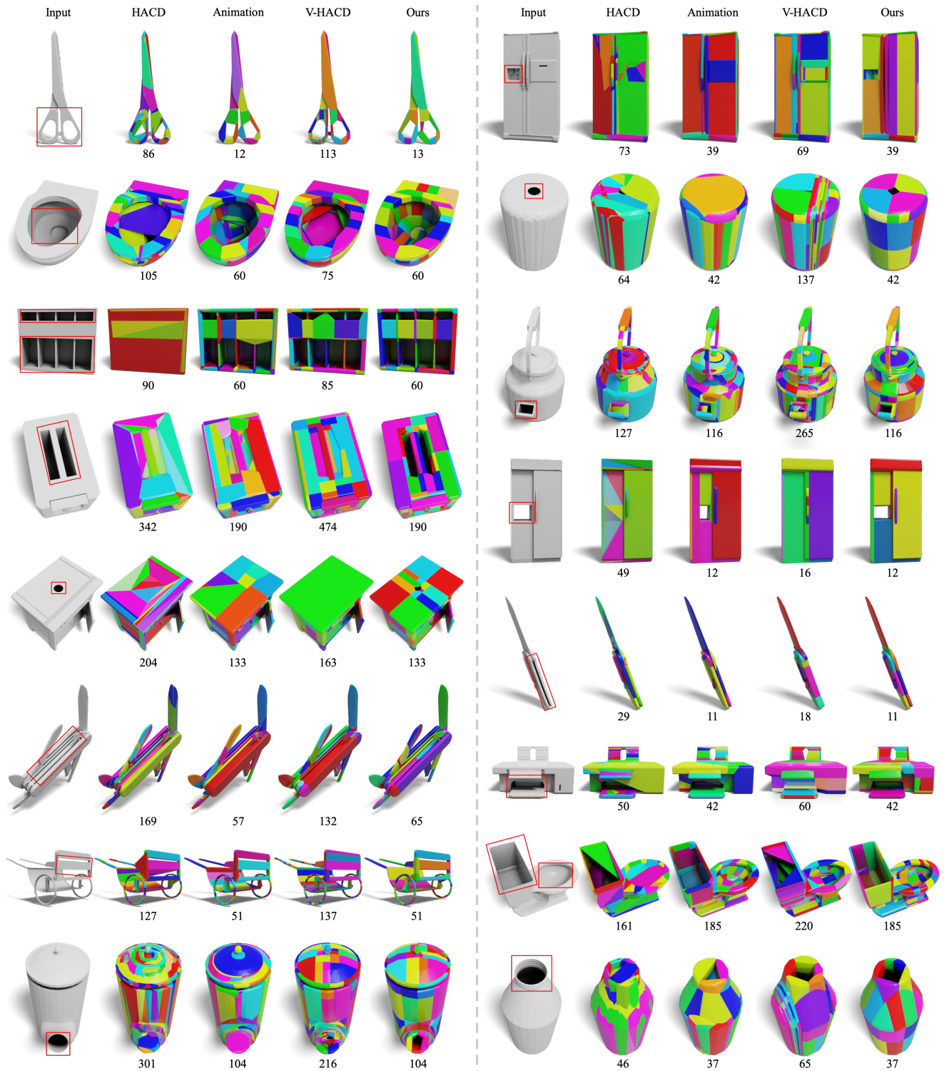
Fig. 11. We compare our method with HACD, Animation, and V-HACD. Please zoom in for the details. The input shapes come from the PartNet-Mobility dataset. Each shape may consist of multiple parts (e.g., two blades of a scissor), and each part is decomposed individually. The red rectangles on the input shapes highlight the error-prone regions. The numbers below the results indicate the number of decomposed components. For both HACD and V-HACD, we set parameters to encourage fine-grained decomposition. For our method, we use a concavity threshold of 0.05. For Animation, we let the number of decomposed components equal our results.
