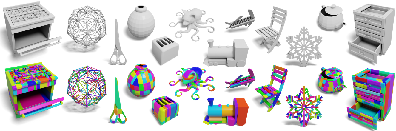
Fig. 1. We decompose a solid mesh into a set of components and utilize the convex hulls of the components (shown in different colors) to represent the original shape. Compared to prior works, we can better capture the fine-grained structures of the input shape with fewer components. See handles of the oven and the cabinet, slots of the toaster, and the spout of the kettle (zoom in for details). The high-quality decomposition enables delicate object interaction in downstream applications (e.g., a robot opens the drawer by grabbing the handles).
