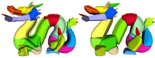
Figure 2: ACD provides a simpler representation of the dragon model using the convex hulls (slightly separated) of its components.
