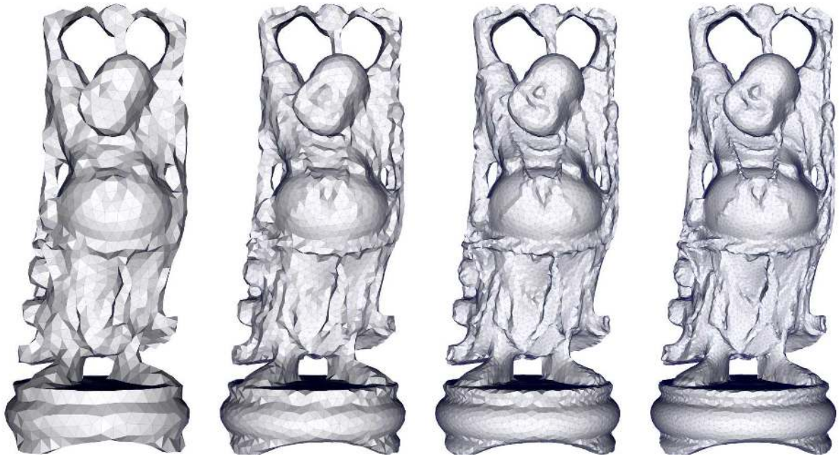
Figure 6: Several coarsened versions of the Happy Buddha model, with respectively 2k, 5k, 10k and 15k vertices.
