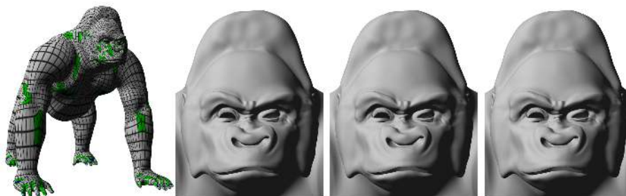
Figure 12: A complex mesh with boundary. From left to right: Catmull-Clark patch structure, Geometry patch approximation, Geometry/Tangent patch approximation and Catmull-Clark limit surface.
