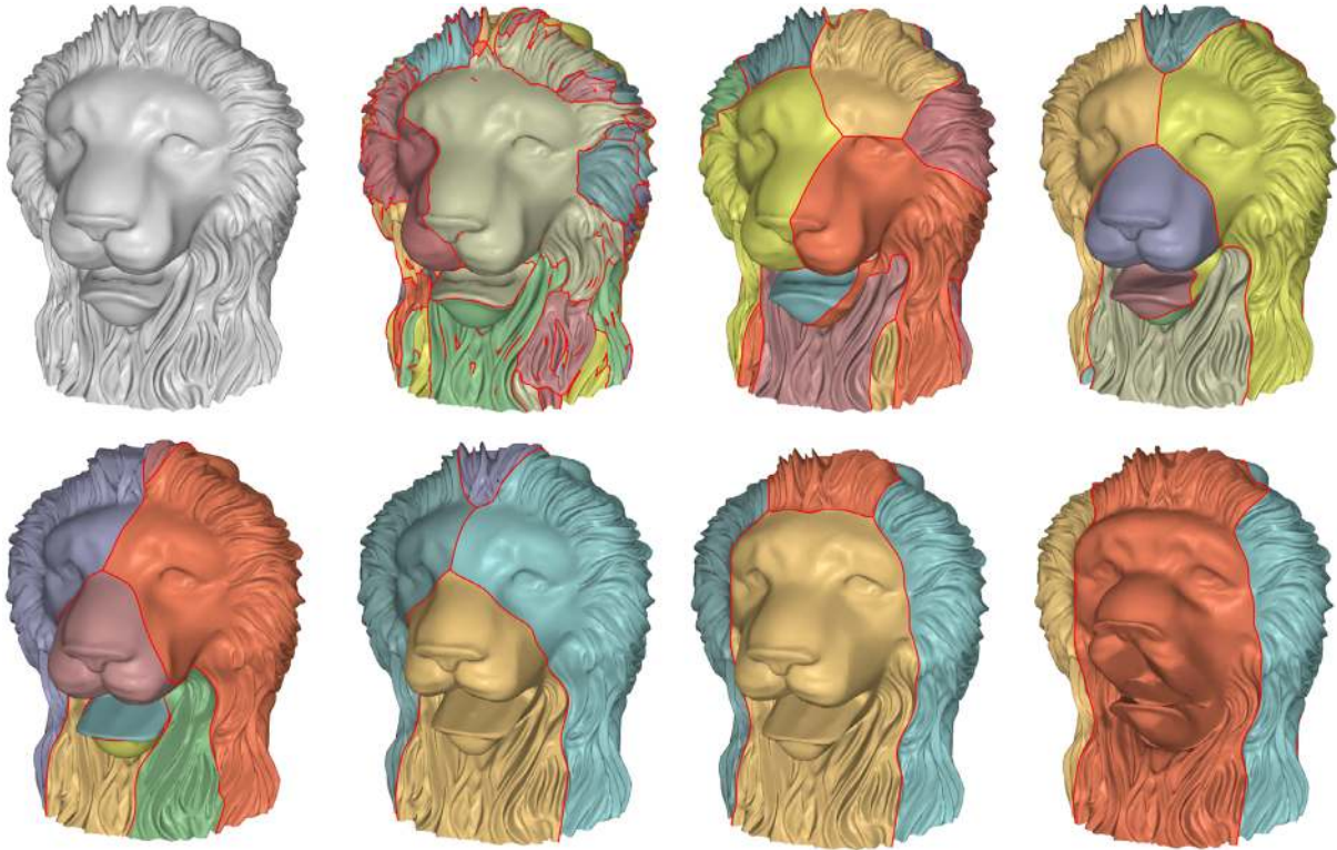
Figure 11: Several instances of segmented meshes for \gamma = 0, 0.001, 0.005, 0.01, 0.05, 0.1, 0.2 . By varying \gamma we can control the number of faces that violate (CI). A value of zero yields no constraint violation (top, center left). Consequently many segments are generated. Choosing \gamma to large yields to much deformation (bottom, very right).
