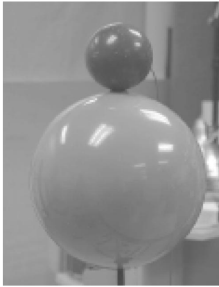
FIG. 2. The physical snowman model, which is composed of a 4.15-cm-radius bocce ball resting on top of a 10.9-cm-radius bowling ball. The probe tube microphone is inside the bocce ball, with the probe tip flush with the surface. The bowling ball is supported by a 0.5-cm-radius cylindrical rod.
