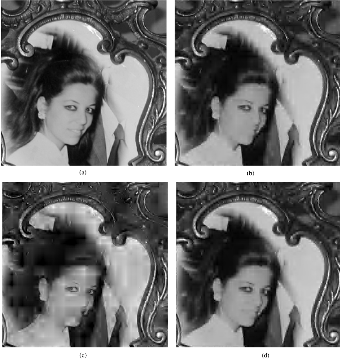
Fig. 3. Representing an image using the optimal strategy that minimizes the \ell_2 error, and our greedy approximation algorithm under the \ell_\infty and \ell_1 error measures. The Daubechies D_2 wavelet is used in all three representations, and the number of retained coefficients is B = 4096 . (a) The original image. (b) Output of the optimal \ell_2 algorithm (which retains the largest B wavelet coefficients). (c) Output of our greedy algorithm under \ell_\infty . (d) Output of our greedy algorithm under \ell_1 .
