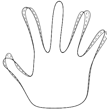
Fig. 12. The result of the Hausdorff warping of two hand silhouettes. The two hands are represented in continuous line while the intermediate shapes are represented in dotted lines.
