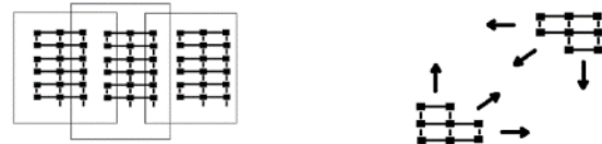
Fig. 21. The distribution of function values in three vertical stripes into three threads (left), the distribution of function values into two triangular regions (two threads) starting from two opposite corners of the domain (right)
