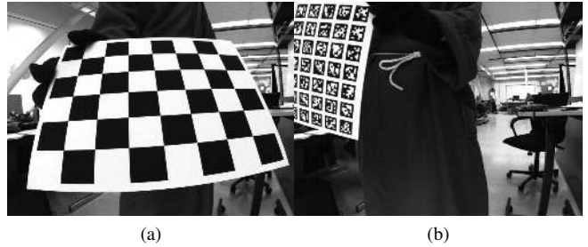
Fig. 3: Example images taken by the participants for both Method A (Open CV) and Method B (AprilCal).
