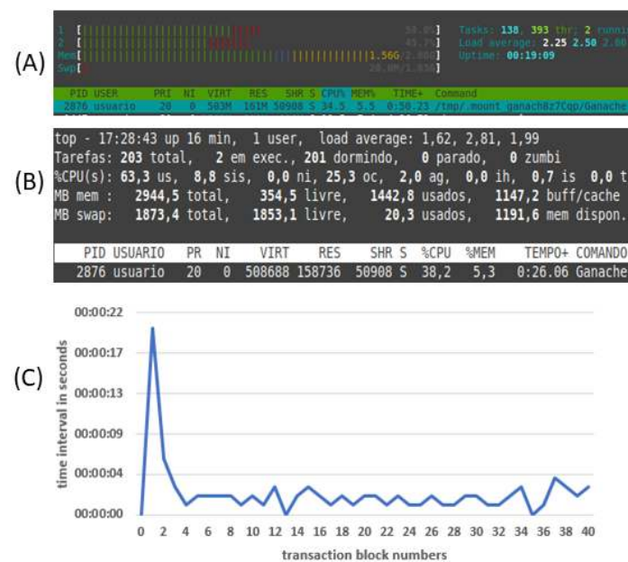
Figure 14. Figures (A) and (B) show top and htop indicating CPU time and (C) transaction time in Ganache at layer 2.
