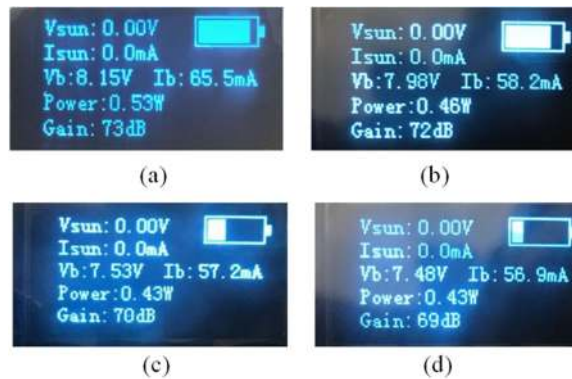
Fig. 6. Photos of the display screen on the receiver circuit of AquaE-lite at the PGA gain of (a) 73 dB, (b) 72 dB, (c) 70 dB, and (d) 69 dB, which show the output voltage ( V_{\text{sun}} ) and the current ( I_{\text{sun}} ) of the monocrystalline Si solar panel for energy harvesting, the total consumed voltage ( V_b ) and current ( I_b ) of the two batteries on the receiver circuit of AquaE-lite, the power consumed by the receiver circuit of AquaE-lite (Power), and the PGA gain values (Gain).
