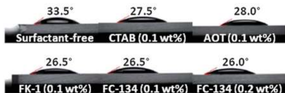
Fig. 11 CA measurements of different aqueous electrolytes at the surface of dye-coated \text{TiO}_2 films. Adapted and reprinted from ref. 163.
