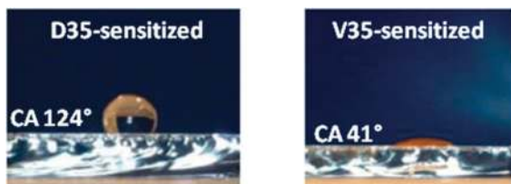
Fig. 19 Crossed sections of working electrodes sensitized with D35 (left) and V35 (right) with a drop of deionized water positioned on the top. CA values are also reported. Adapted and reprinted from ref. 249.
