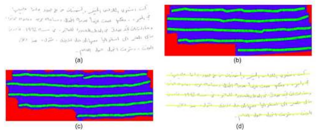
Fig. 8. Results of text-line segmentation: a) the original image, b) the ground truth composed of three classes (background: red; paragraph: blue; x-height: green), c) the output of the RU-net, d) the final result after post-processing.
