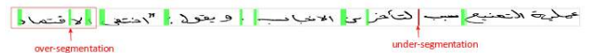
Fig. 12. Example of wrong segmentations. The red box denotes one word and an over-segmentation is made on the sub-words.
