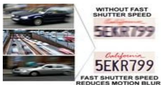
Fig 2. Results from camera with/without improved shutter speed, (B) LP (Guangming Li, et al, 2010)
