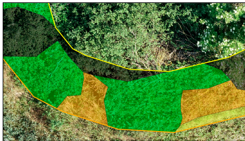
Figure 2. Cutout of the vegetation growing at the edge of one kettle hole investigated in 2019/2020. Image collected by an Unmanned Aerial System (UAS) in June 2020. Orthomosaics were created with this image by using Agisoft Metashape Professional 1.6.2 build 6205.
