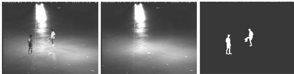
Fig. 11. An example of background subtraction. (a) Input image, (b) background image, and (c) background subtracted image.
