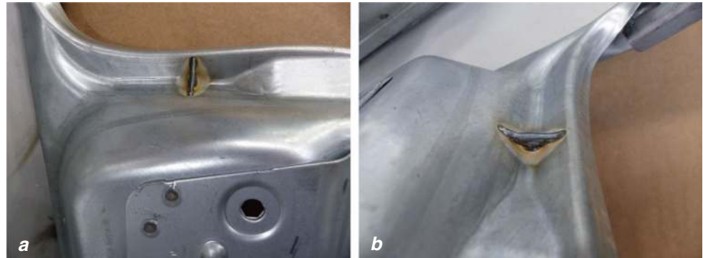
Fig. 10 a, b Welding results of additive manufacturing of a gusset plate on car body area of 0.7 mm thickness
