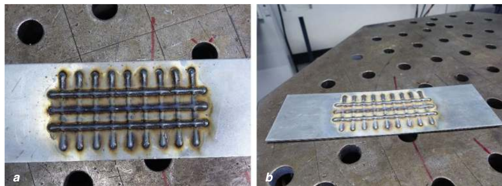
Fig. 8 a, b Welding results of additive manufacturing a grid on zinc-coated steel sheets of 2 mm thickness
