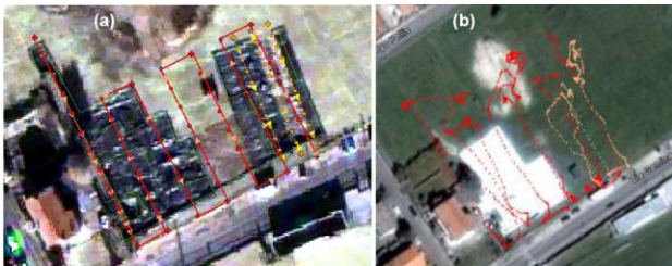
Figure 4. The flight planning on the Quickbird orthophoto (a) and the real trajectories followed by the aircraft (b): red lines described the highest flight and orange lines the lowest flight
