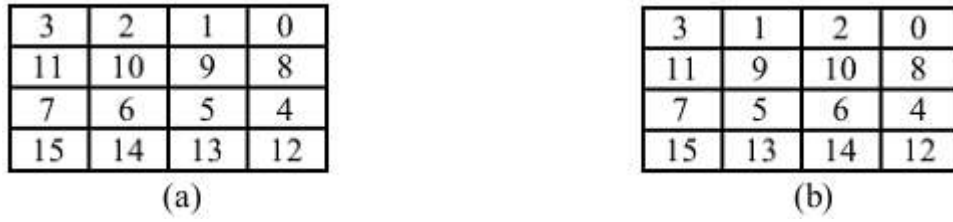
Figure 6.6. Data flow order in the proposed architecture of (a) inputs and (b) outputs
