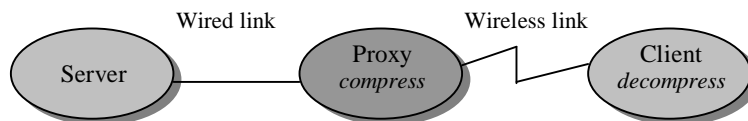
Figure 1: Use of a proxy to reduce bandwidth requirements over a wireless link.
