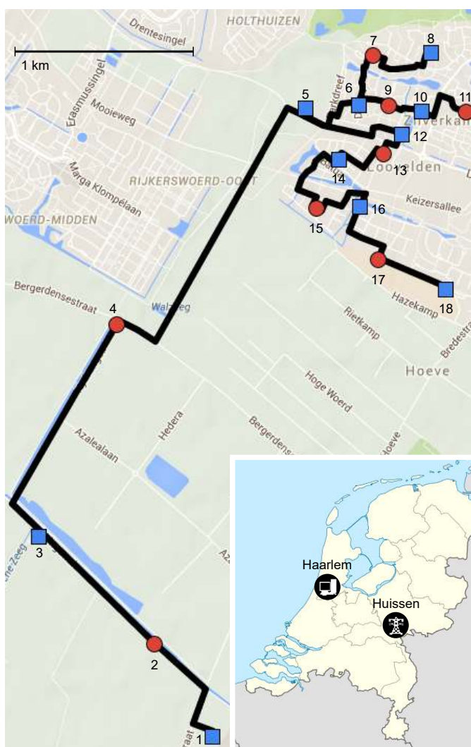
Fig. 7. Network topology of the Alliander 10 kV feeder showing the PMUs and PDC locations.
