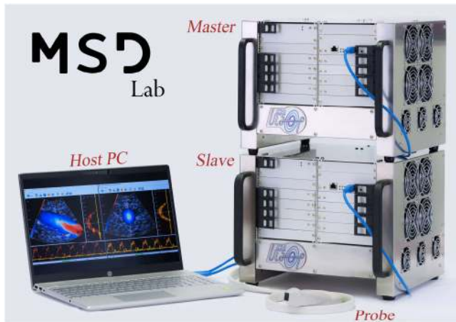
Fig. 3 The 512-channel demonstrator.
