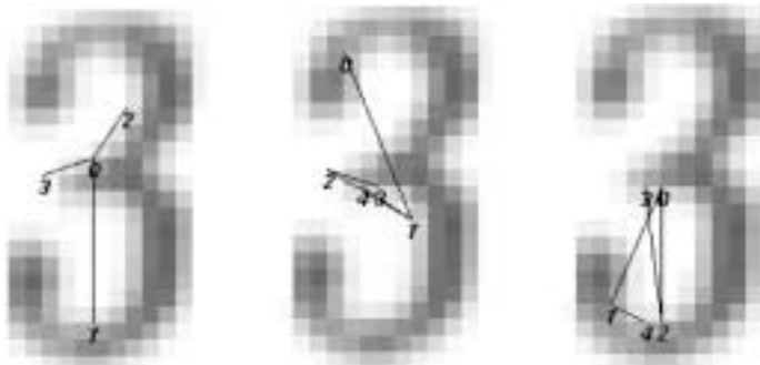
FIG. 1. The arrangement found on a sample “3” in three different trees. The lines connect pairs of points for which the relative orientation is defined in the arrangement.
