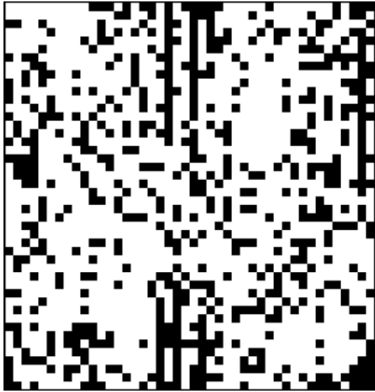
FIG. 10.—Results of beam mapping the ARCONS array. Pixels with good locations are shown in white. Vignetting is apparent at the bottom right side of the array. The overall pixel yield in this engineering-grade array is \sim 70\% .
