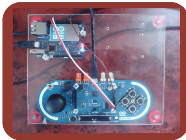
Fig. 5. Esplora & Yun board serial connection
