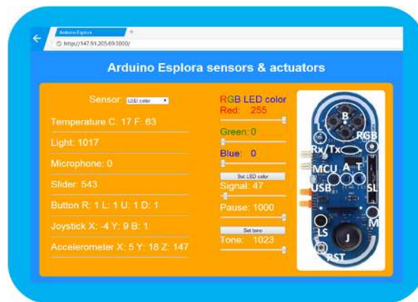
Fig. 6. Web page with Esplora sensors and actuators
