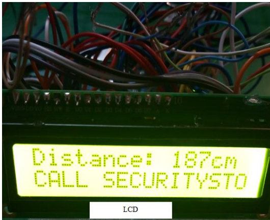
Fig. 6. A motion detector with display of distances on the Liquid Crystal Display.
