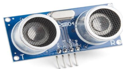
Fig. 1. Ultrasonic sensor for ultrasonic wave production in motion detection.
