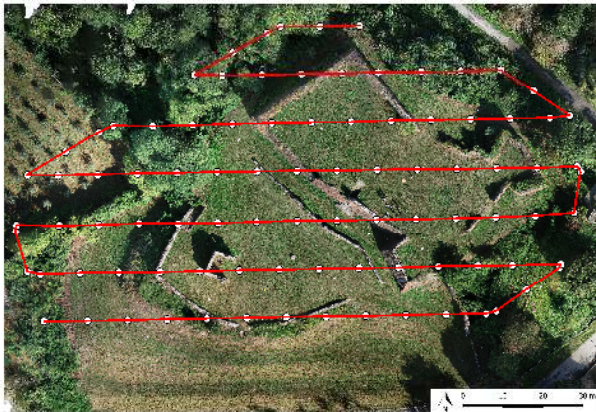
Figure 3 Flight plan for Castellazzo area. Flight lines in red and camera positions highlighted with white dots.
