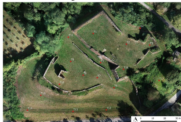
Figure 1 (a) Distribution of the control points measured on the test site (red dots).
