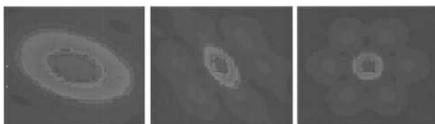
Fig. 12 PSF plots when the beam combiner has tilt errors. From left to right, X tilt: 0.2, Y tilt: 0.4; X: 0.3 Y: 0.3; X: 0.25 Y: 0.25 (deg).
