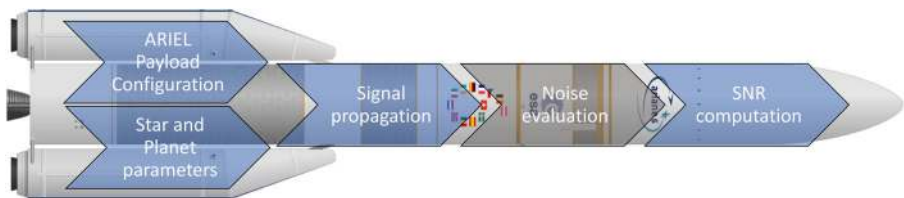
Fig. 1 Simulator work flow. The simulation starts with two input files: a payload configuration file and a candidate planet list. ArielRad propagates the target host star signal through the payload, then evaluates the noise. Finally, the simulator estimates the transit or eclipse observation and the resultant SNR
