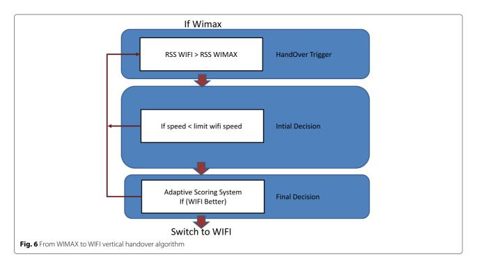
stage, an adaptive scoring system reads multiple parameters to decide which network is the best according to the user preferences. If the scoring system decides that WIFI is better than WIMAX, then vertical handover occurs.
