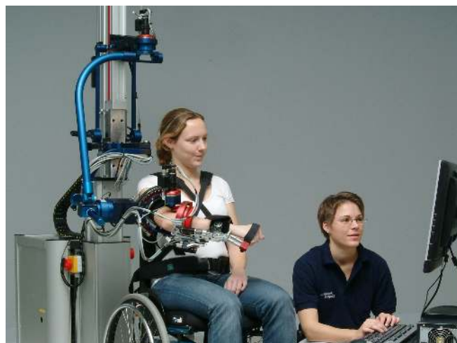
Fig. 5. Subject sitting in a wheelchair is coupled to the ARMin II robot. A physiotherapist sitting near by is selecting the rehabilitation procedure.
