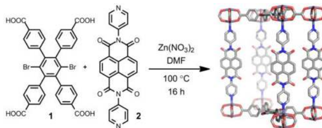
Scheme 2. Synthesis of Noninterpenetrated Br-YOMOF
