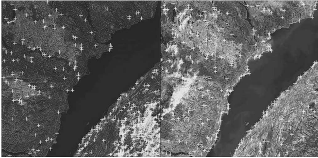
Fig. 1. Extracted CP candidates (as indicated by crosses). (Left) Reference image. (Right) Sensed image.
